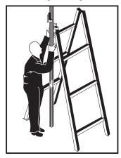
6. Fit speader bar with trestle in fully open position. Make sure steel tongue fits up into the slot provided in "Master Post". Tighten handles.
